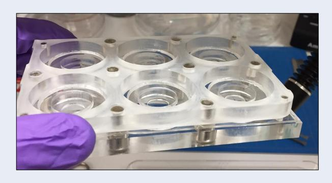
Figure 3. Image of the 6 well plate used in bioreactor with PDMS pillar membrane.
