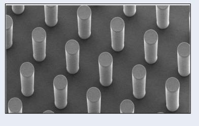
Figure 1. Scanning electron microscope image of micropillars approximately 200µm in height and approximately 75µm in width [4].
