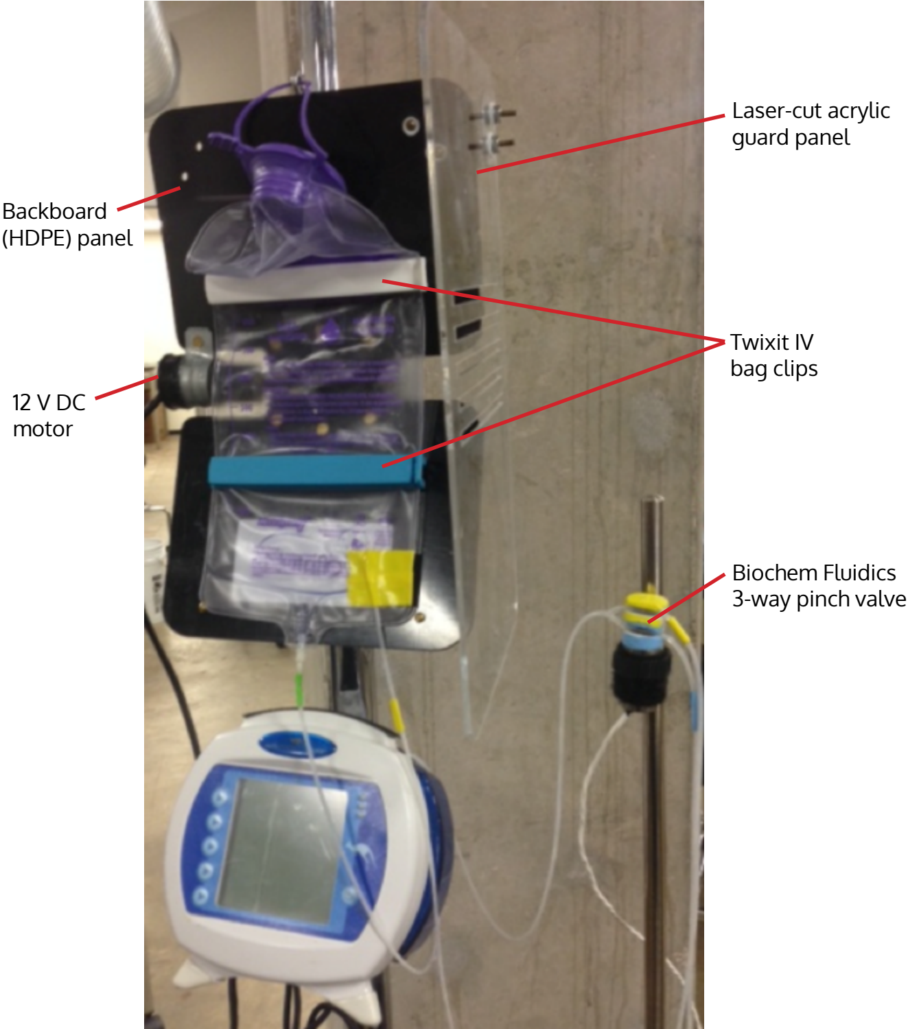
Labeled Nutriflow device without additional bypass pump attached
